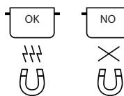
Only use pots and pans made from ferromagnetic material which are suitable for use with induction hobs:
