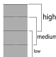
The flexible zone is divided into three cooking zones (see the figure) activated at a pre-set power (high, medium or low) depending on the position of the pot/pan: move the pot/pan over the surface to continue cooking at different temperatures without having to use the controls.
